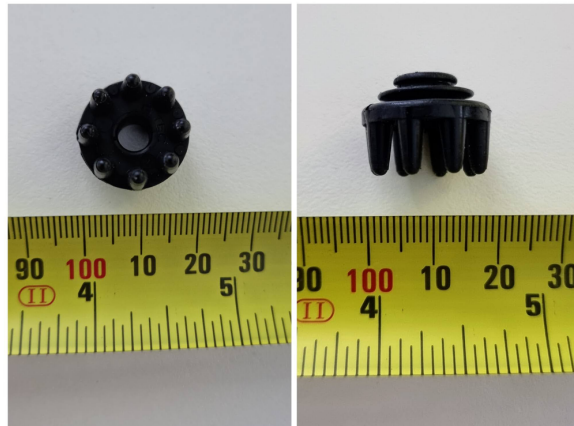
Figure 5: Electrodes supplied with the g.tec Unicorn Black BCI may have had some impact on the EEG signal stability in participants with long hair.
